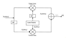
Fig .2 Illustration of OSSB modulation using phase shift method
