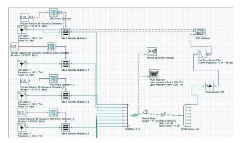
Fig .3 Simulation Setup of WDM
