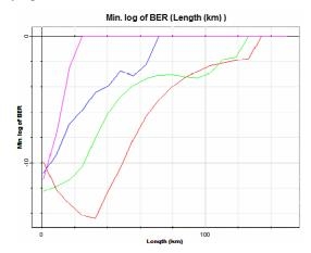
Fig .6 BER plots for all the four channels in SCM
